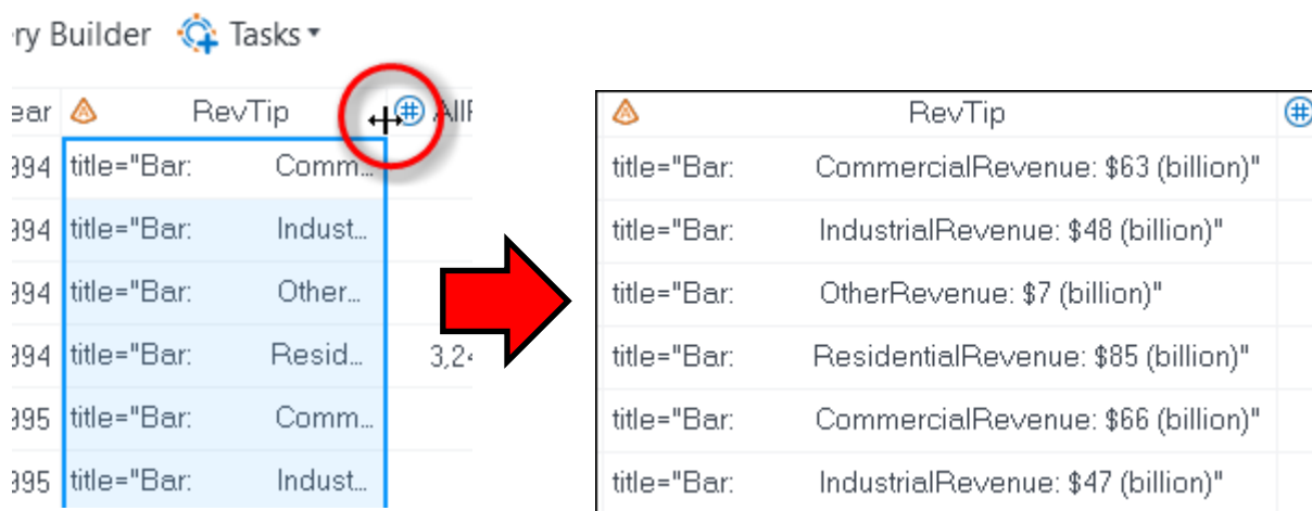
Figure 13: Resizing a Column
