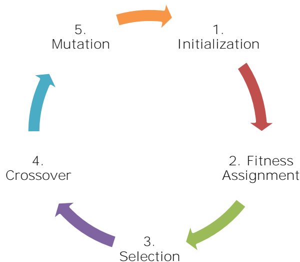
Figure 2: Evolutionary Cycle of Feature Selection.
