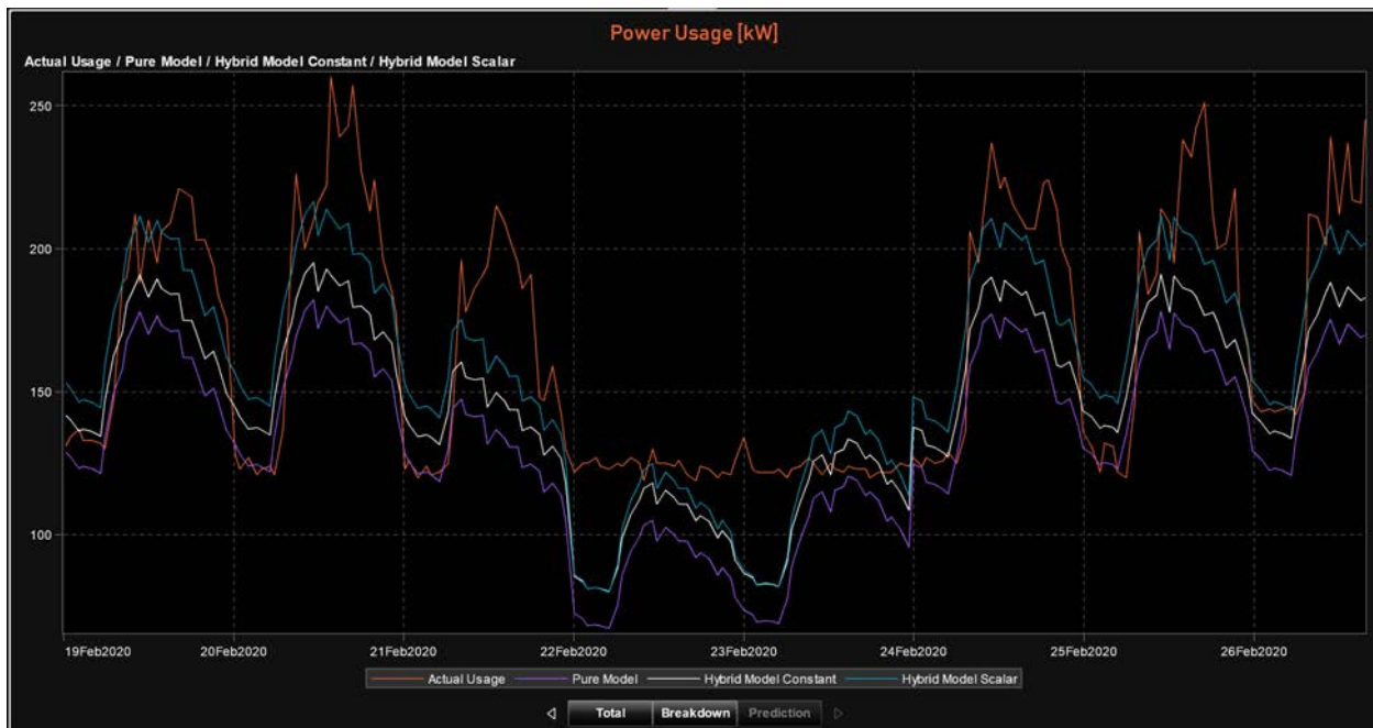
Figure 7. Watt Center Power Forecast Model for February 19, 2020 to February 26, 2020; Legend: Red = Observed, Purple = NN, White = Hybrid Constant, Blue/Green = Hybrid Scaler
