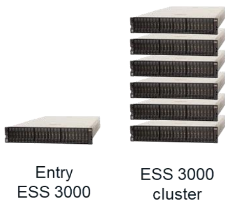
Figure 3. Elastic Storage Server scales out by adding 2U drawers
