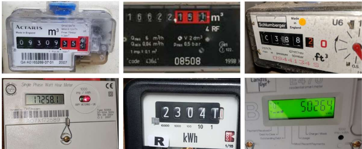
Figure 3. UK Gas (Top) and Electricity (Bottom) Meters
