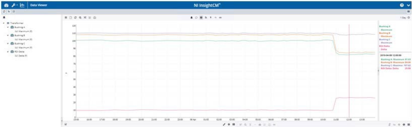
Figure 2. SAS Event Stream Processing monitoring the temperature of bushings on a transformer to determine at what rate the transformer is being used
