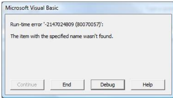
Figure 4 Error message because "Chart 1" may not exist when the macro runs. A second execution may produce "Chart 2".
