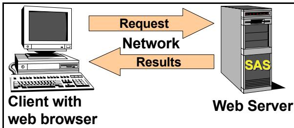
In fact, web-based configurations can be quite complex, with separate servers for both SAS Software and databases.
