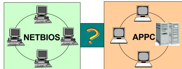
The Domain Server can act as a protocol gateway between network segments that use different protocols. Only one machine in the network needs to have both protocols installed.
