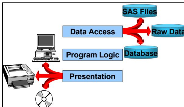
In a single-platform application, all components execute on the same computer. In a client/server application, you can choose among multiple computers for each functional component:
