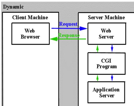
“CGI (Common Gateway Interface)” is a programming interface that allows a web server to communicate with an external program. CGI programs are typically small, written in a script or high level language and reside on the web server to act as an interface between a web browser and a database server or application server<sup>1</sup>.
