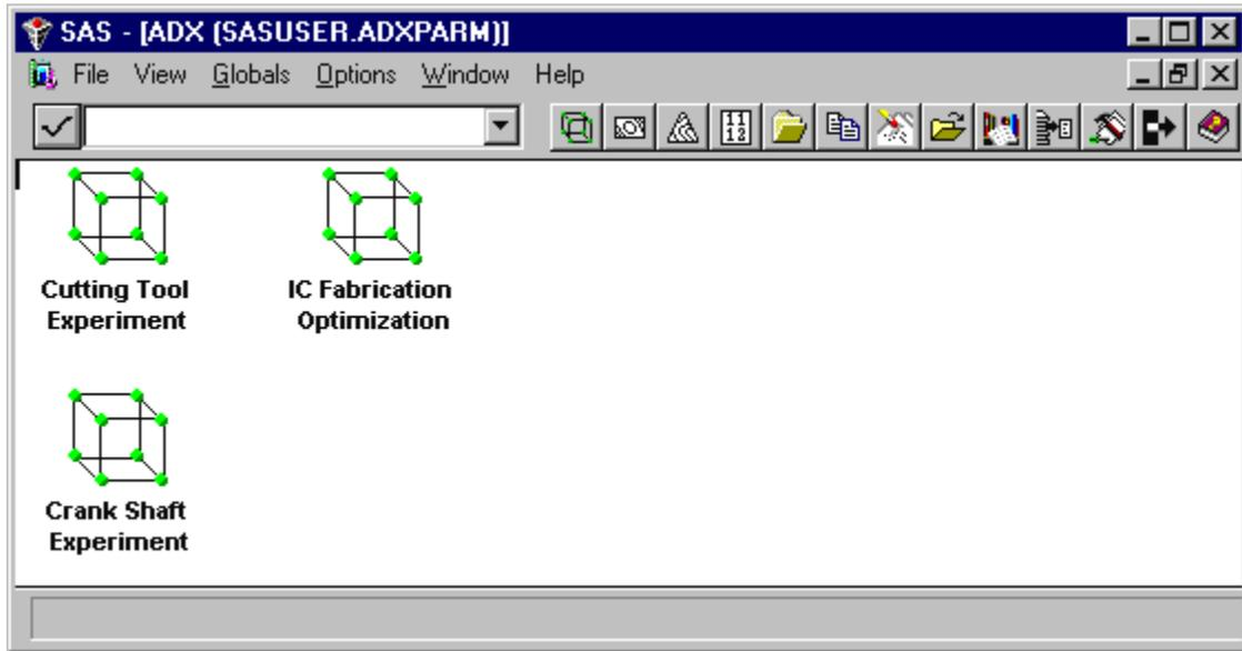
When you invoke the ADX interface you first see the ADX desktop with the icons representing any designs that you previously constructed and saved. The ADX desktop provides a placeholder to organize and view the designs. You can copy a design, view a design summary, or export a design to a data set from the desktop. The following example illustrates how a design is constructed and analyzed using the ADX interface.
