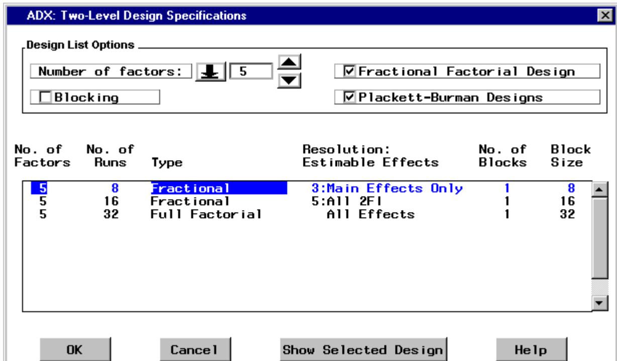
To examine the characteristics of a design, double-click a design row in the list. For instance when you point the mouse to the five-factor design in 8 runs and double click, you see the design details as displayed in the following screen.
