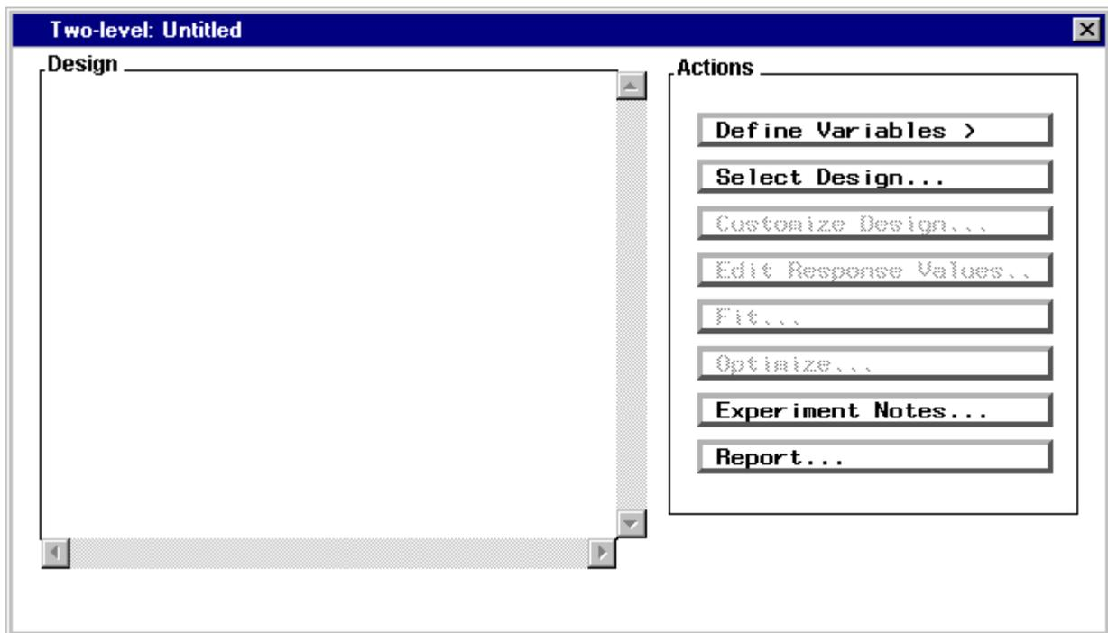
To begin specifying a new design, you can either enter factor names and levels or select a design. When you press the **Define Variables >** button and select **Factors and Levels...** item you get the Factor and Block definition screen.
