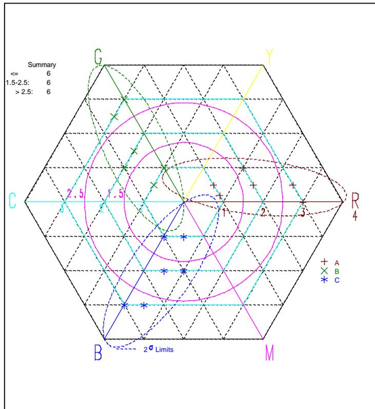
This is a kind of graphic we use at Kodak to evaluate the color balance of photographic materials. We wanted the ability to generate such a graph within the SAS® System, as part of a researcher's or engineer's analysis. None of the standard SAS/GRAPH procedures could easily produce this, however. Our solution was to write a DSGI program.
