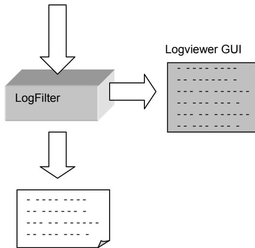
The Logviewer plugin intercepts the standard logging stream, and writes its contents to both the viewer window and to the file for which it was originally destined. (In the process, it corrects a “quirk” in the format of the log stream to ensure that the log contents has OS-appropriate line breaks – the normal log is not legible for Windows clients.)
