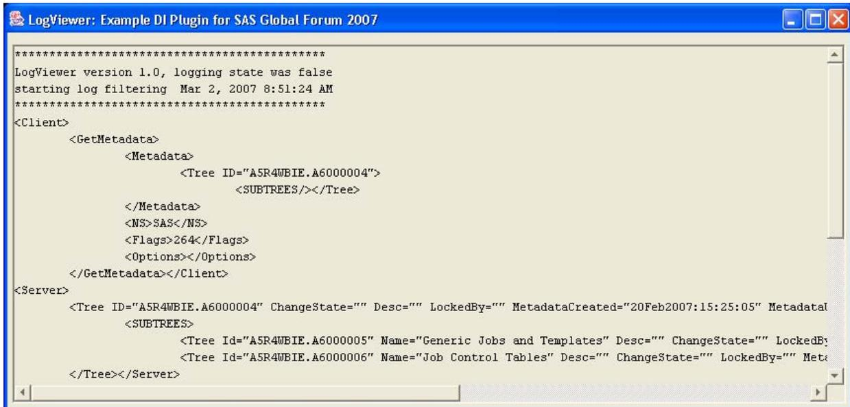
When you interact with SAS Data Integration Studio's interface, the metadata conversation between the client and the server appears in the window. Above, we see the query and response from opening a Tree with the ID "A5R4WBIE.A6000004." The server responds with a list of subtrees, one named "Generic Jobs and one named Templates" and "Job Control Tables."
