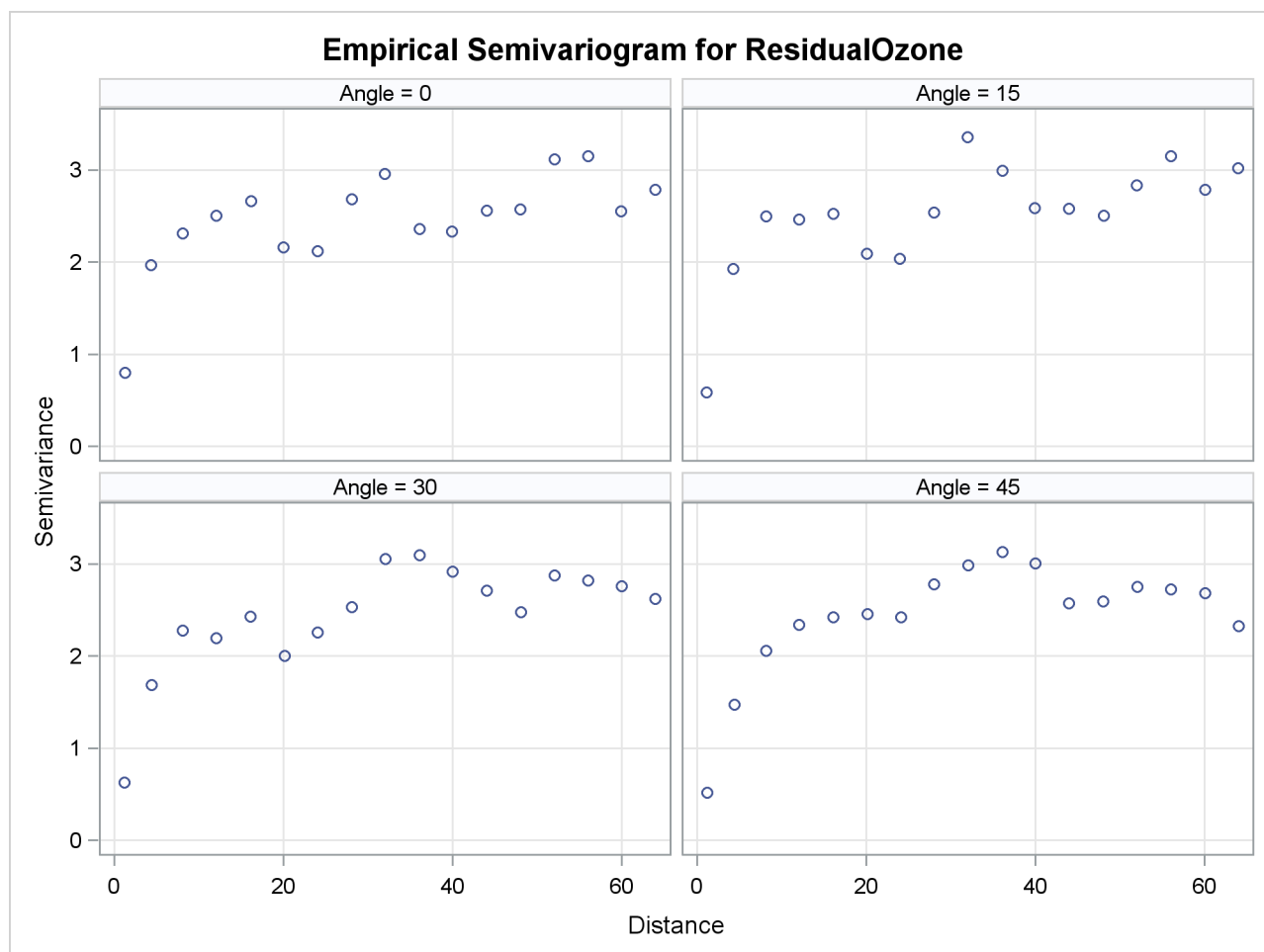
Output 122.2.6 Ozone Empirical Semivariograms with 0^\circ \leq \theta < 180^\circ and \delta\theta = 15^\circ
