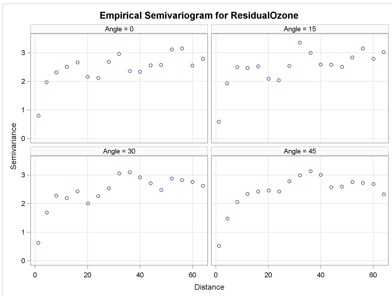
Output 109.2.6 Ozone Empirical Semivariograms with 0^\circ \leq \theta < 180^\circ and \delta\theta = 15^\circ
