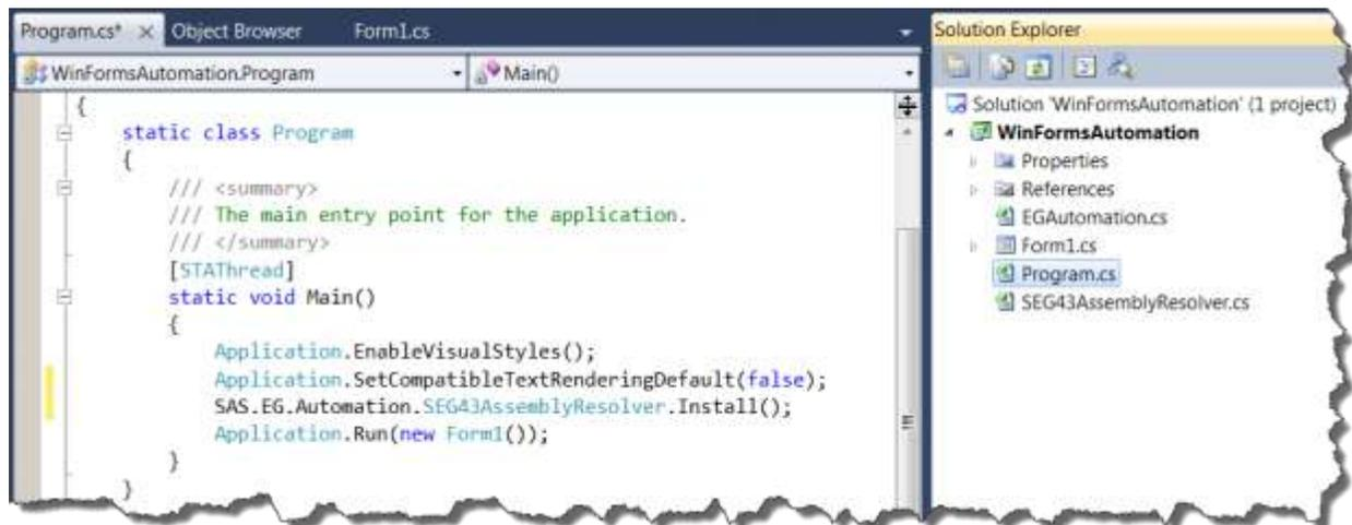
**Figure 4. Helper Classes and Assembly Resolver Function Call**
