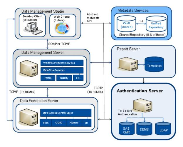
The DataFlux Authentication Server is required in all deployments that include a DataFlux Federation Server. Otherwise, the Authentication Server is optional. Your deployment may include more than one Authentication Server.
