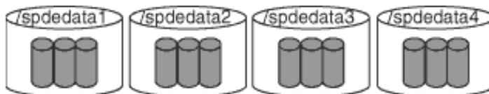
Figure A1.3 Four RAID 5 Arrays, Each Striped across Three Disks
