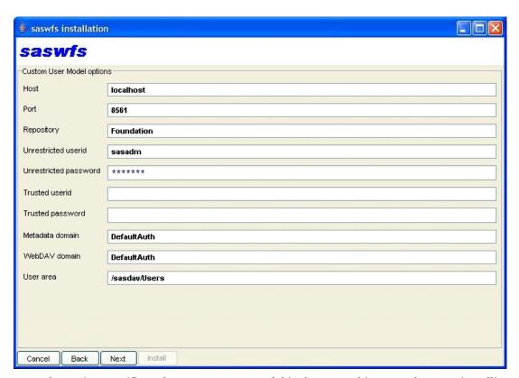
3. Information specific to the Custom User Model is shown on this page. If you are installing Xythos as part of a planned install, this information should be the same as that already specified in the Configure Wizard. The trusted userid and password are only required when the metadata domain and WebDAV domain are different. More information on these values can be found in the "Custom User Model" section, beginning on page 8.
