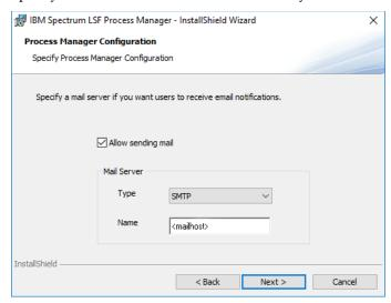
The email configuration is optional. If you do not want IBM Spectrum LSF Process Manager or IBM Spectrum LSF to send email notifications, leave the check box cleared.
