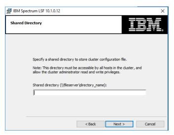
**Note:** Make sure that the Primary LSF administrator account (such as <domain>\sas) has Write permission to the network share. Otherwise, you will receive Error 30035 about the failure to run the egoconfig mghost command.
