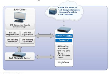
Job scheduling on a single machine requires you to install IBM Spectrum LSF Process Manager for SAS. During the IBM Spectrum LSF Process Manager for SAS installation, you also install IBM Spectrum LSF for SAS. See "Chapter 2 - Installing IBM Spectrum LSF Process Manager for SAS and IBM Spectrum LSF" for the instructions on installing on a single server.
