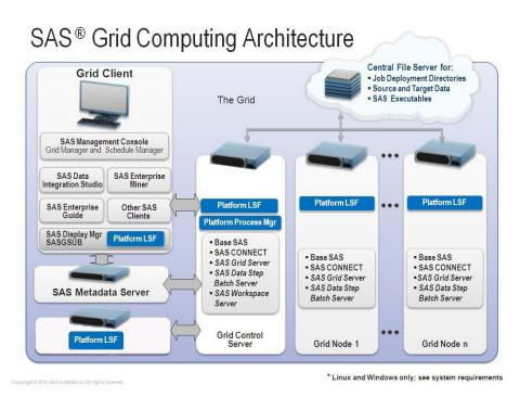
Several types of machines make up a SAS grid environment. These machines have been defined to clarify the software components that must be installed on each one as well as the SAS metadata that must be configured. The SAS Metadata Server is shown on a separate machine in this example architecture. It is common to dedicate a machine to running the SAS Metadata Server, but you might instead choose to run the metadata server on the grid control server.
