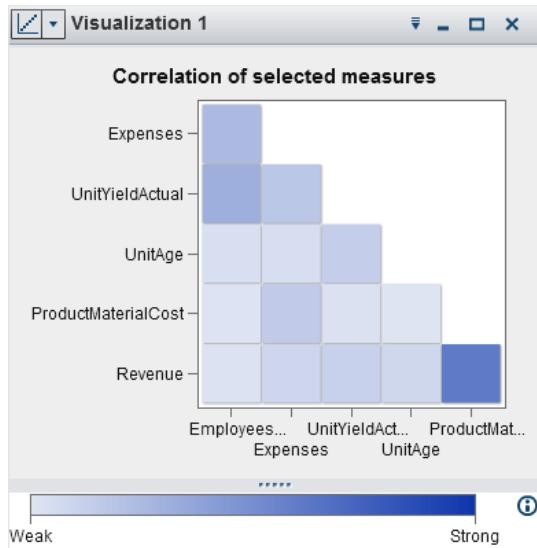
A correlation matrix displays the degree of correlation between measures as a series of colored rectangles. The color of each rectangle indicates the strength of the correlation.
