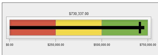
A bullet gauge is a dashboard indicator (also known as a key performance indicator (KPI) chart) that compares an actual value to a target value in intervals. This example displays three bullet gauges. The actual value is indicated by an inset bar.
