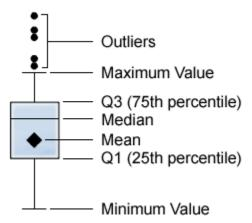
Figure 20.3 on page 169 shows a diagram of a box plot. The bottom and top edges of the box indicate the interquartile range (IQR). That is, the range of values that are between the first and third quartiles (the 25th and 75th percentiles). The marker inside the box indicates the mean value. The line inside the box indicates the median value.
