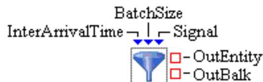
Figure 4.2 Entity Generator Block with Five Static Ports
