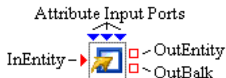
Figure 4.3 Modifier Block with Three Dynamic Attribute Ports
