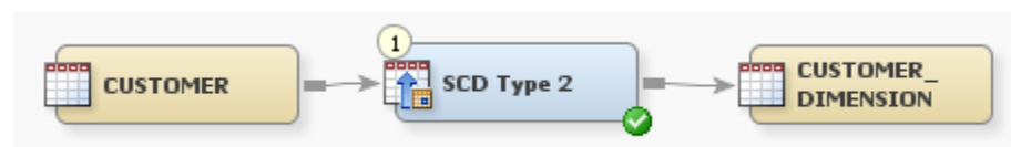
Display 19.2 Sample SCD Type 2 Loader Process Flow Diagram
