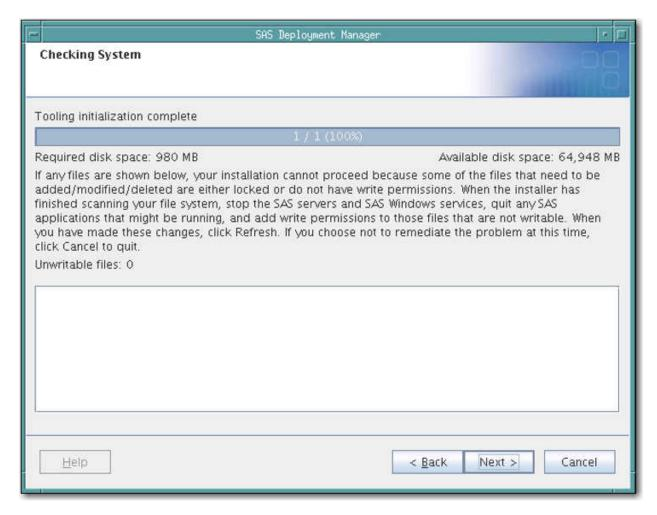
**14** If any files are shown in the text box after the system check, follow the instructions on the **Checking System** page to fix any problems.
