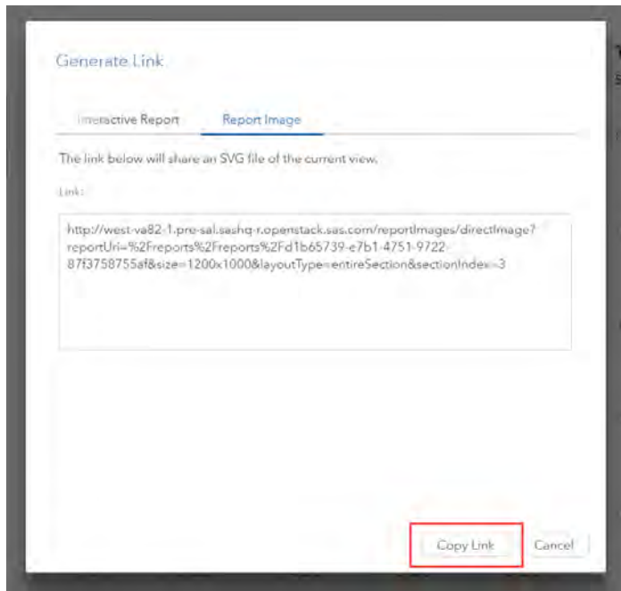
Figure 21. Embedding and Sharing Reports and Report Objects – Using the share options on a report or report object, you can generate a call to the default API provided out of the box.
