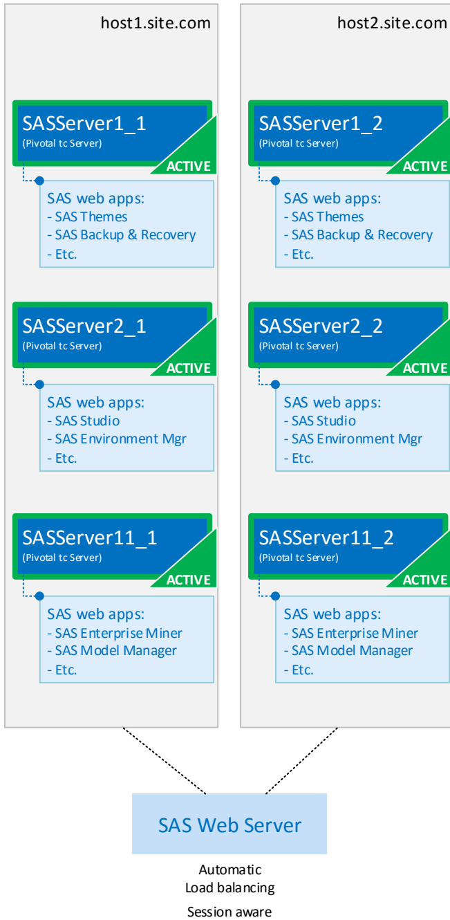
Figure 5. The SAS Web Application Server with JVMs Clustered Both Vertically and Horizontally
