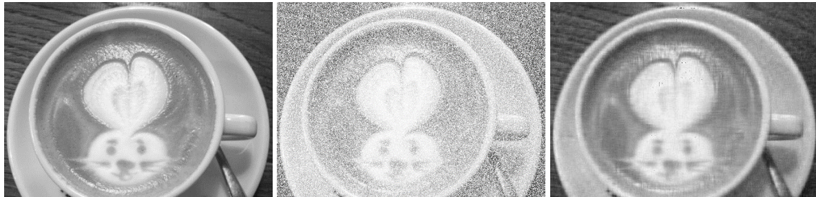
Figure 5. Image reconstruction. Left: Original image. Center: 50% missing pixels. Right: Image reconstructed using PROC FACTMAC.
