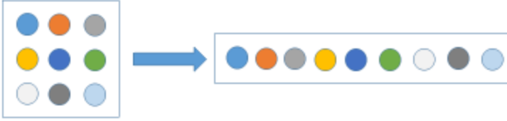
Figure 2. Example of patch vectorization. Pixels are rearranged in a row vector in lexicographic order.
