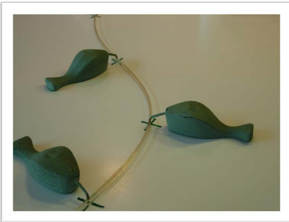
Figure 1. A draftsman's spline, with ducks. Used with permission.
