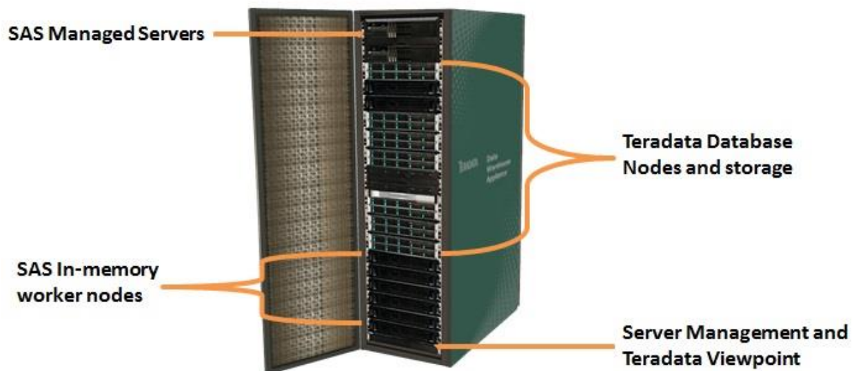
Figure 7. SAS Managed Servers, Data Store, and SAS In-memory cluster "In a Box"
