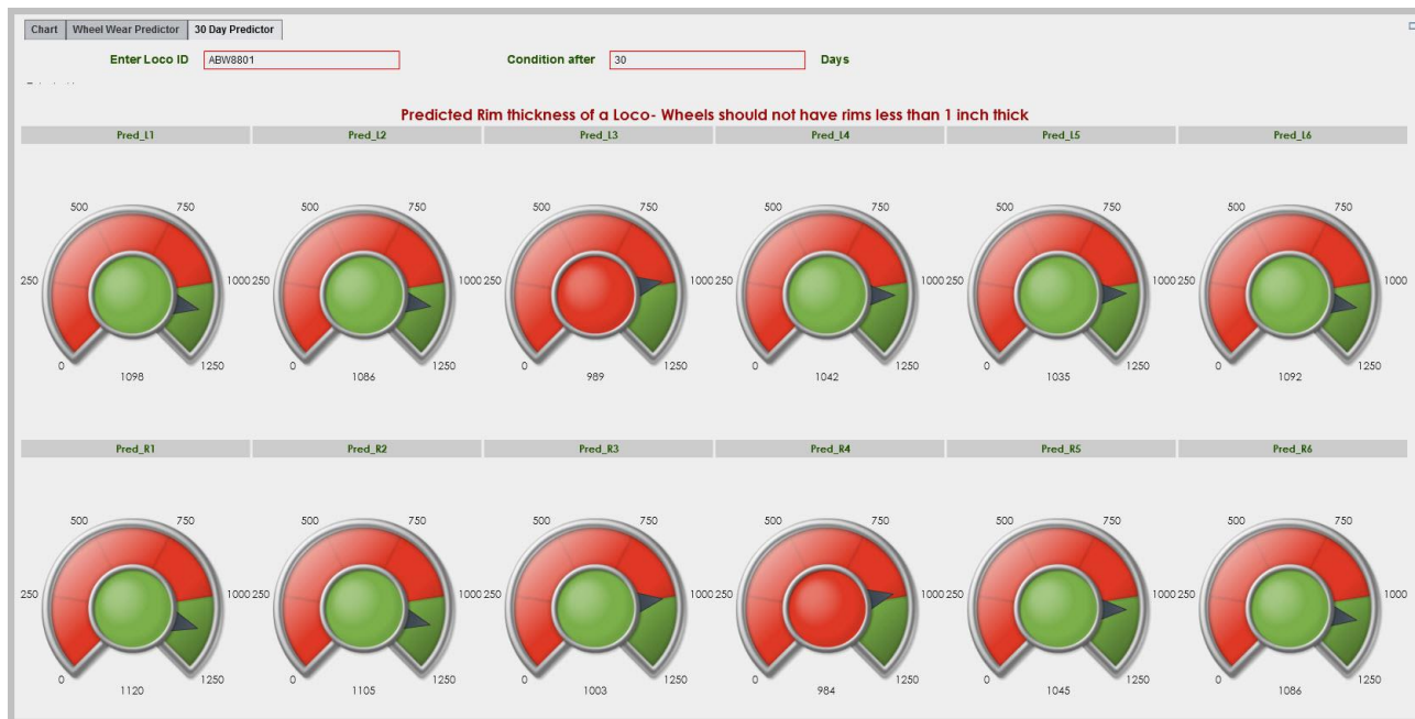
Figure 4 Gauge Display of a Locomotive’s Predicted Rim thickness using “Display Rules”
