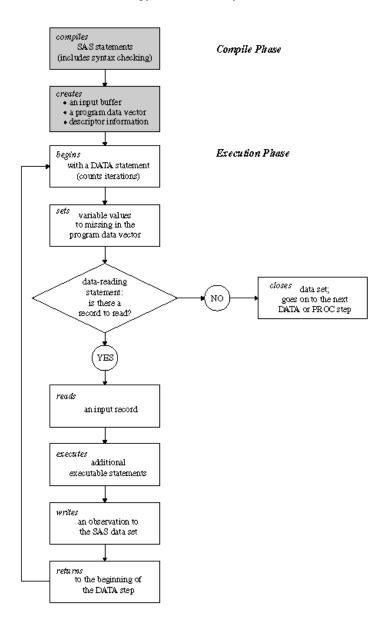
Data step processing diagram from How the DATA step works: A Basic Introduction.
