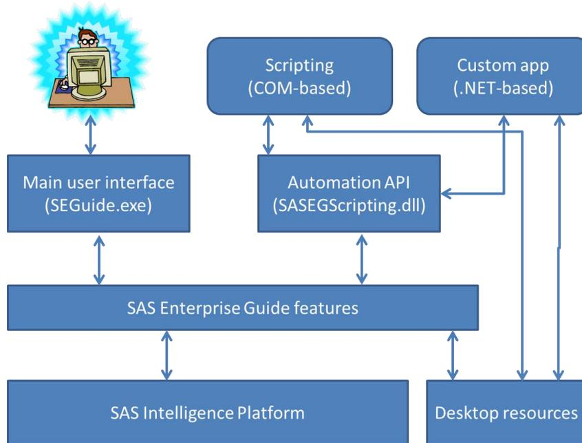
Figure 1. Simple View of the Automation Architecture
