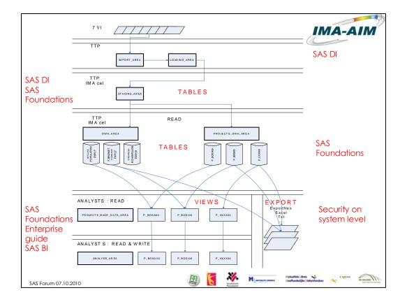
There is one central infrastructure with different environments, for designing, testing and production and the central system is accessed from different location with different networks, security levels and software's.
