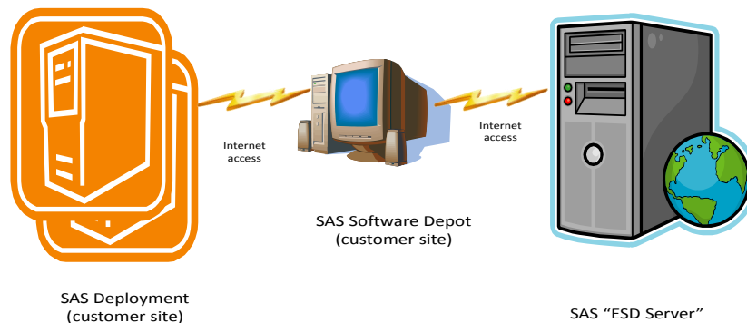
Figure 2: ESD Creates a SAS Software Depot That Is Used To Create or Update a SAS Deployment.
