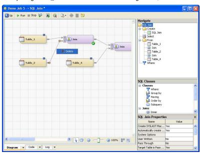
Positioning the mouse near the node causes the cursor to transform into a 4 sided arrow. This tool allows one to move linkages.
