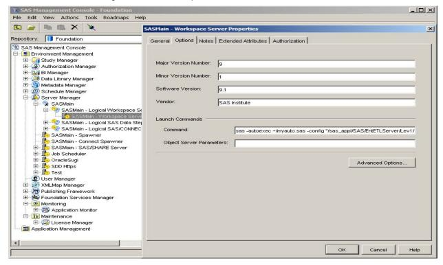
This would allow a per-person inclusion of the autoexec in the logged in users home directory. However, it requires that jobs run from a non-project repository setup to have their own Unix or Windows logins. For jobs run from the Foundation repository you would need a special account to run in production mode versus project mode.
