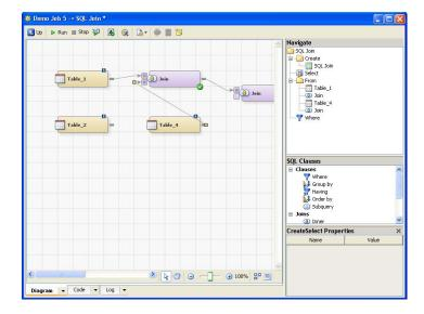
After pulling the linkage from Table\_4 to the first join node, move the cursor towards the right edge of Table\_2, where it becomes a pencil. Using the pencil tool draw the linkage to the second join node. Unfortunately, in the case of left joins, the where-clause statements will not be preserved.
