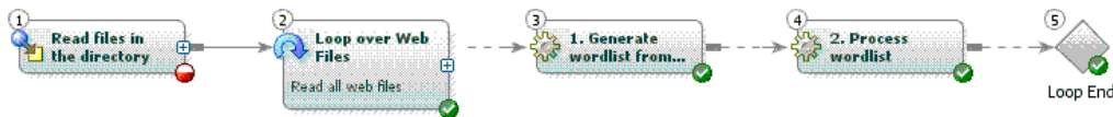
Figure 20. Performing the Text Transforms in Parallel Is Easy Using the Loop transform in SAS Data Integration Studio.
