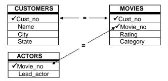
The following SQL code references a join on three tables with CUST\_NO specified as the connecting column for the CUSTOMERS and MOVIES tables, and MOVIE\_NO as the connecting column for the MOVIES and ACTORS tables.
