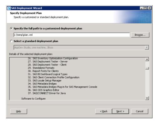
Select the machine. For this example, the **Server** machine is used. Continue on through the pages and upon reaching the **Deployment Summary**, click **Start** to begin the installation process. When the SAS Deployment Wizard finishes, SAS Inventory Optimization and its dependent components will be installed on the selected **Server** machine and are ready to be configured. Restart all SAS servers and spawners and then invoke the SAS Deployment Wizard.
