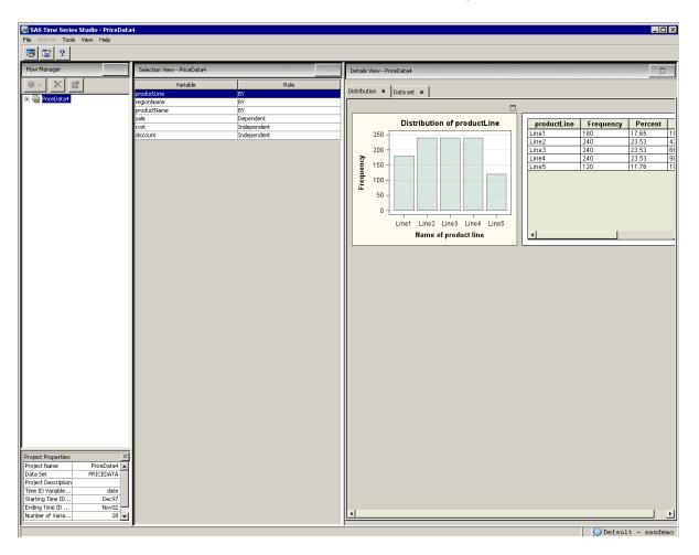
The Selection Manager displays the name and role of each variable in the project. By default, the first variable, productLine, is selected. So in the Distribution tab of the View Manager, you can see a graph of and statistics for the discrete distribution for the productLine variable.
