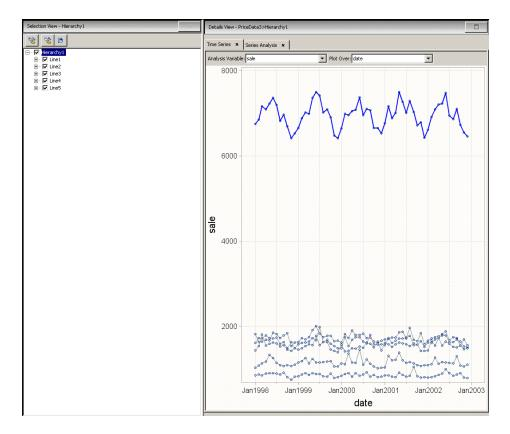
You can also view the data from the levels in the hierarchy. For example, in the Flow Manager, expand the Hierarchy1 node, and you see four levels: Top, productLine, regionName, and productName. The lower that you go in the hierarchy, the more data that appears in the time series graph. By comparing the data from different levels, you can determine how the various "children" impact the aggregation of data at the higher level.
