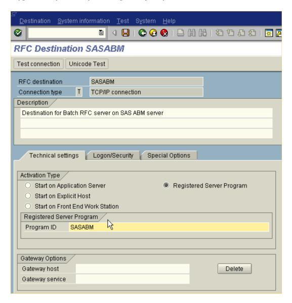
In this example, the destination and program ID are both called SASABM. The connection type must be "T" (TCP/IP connection), and the Activation type must be Registration (Registered Server Program).
