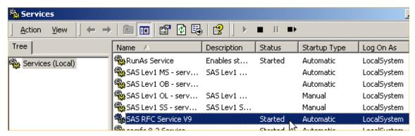
In the Windows services window, check the SAS RFC Service V9 service is correctly started, and is set to start-up automatically.
