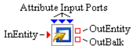
Figure 4.3 Modifier Block with Three Dynamic Attribute Ports
