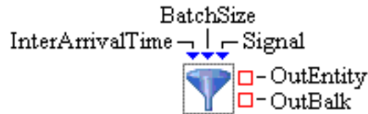
Figure 4.2 Entity Generator Block with Five Static Ports
