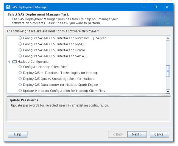
3. Under Hadoop Configuration, select **Deploy SAS In-Database Technologies for Hadoop**.
