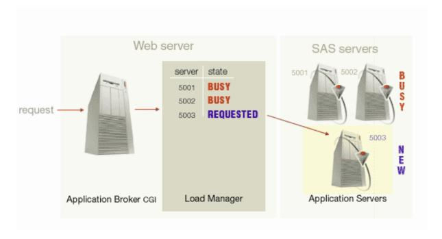
The new server is then added to the pool of servers for that service. The following diagram illustrates how a new server is added to the pool of servers.
