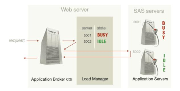
If no servers are free, the request is queued by the Load Manager until a server becomes available or until the time-out value is reached. For pool services, the Load Manager can start a new server to process the request. The following diagram illustrates how the Load Manager starts a new server to process the request.
