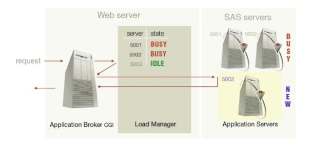
By using a Load Manager to maintain the state of Application Servers, requests are distributed to idle servers. Each Application Server notifies the Load Manager when it starts and completes a job by using the Load Manager socket address that is passed by the Application Broker. This data is used by the Load Manager during subsequent requests to determine which Application Servers are busy and to direct the Application Broker to use an available idle server.
