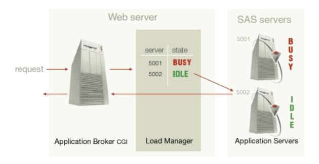
After completing the job, the Application Server again notifies the Load Manager that it is free to work on another request. The following diagram illustrates how the Application Server notifies the Load Manager after it is free to process the next request.
